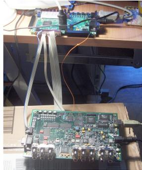
Figure 1: Two demo boards with DSP and FPGA connected.
